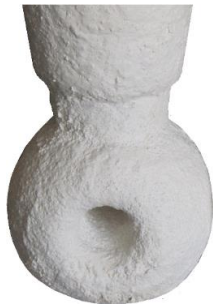
TITANIUM CARBIDE (TiC) POWDER FILLED AND COMPACTED INTO MOLD
