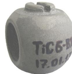
TiC-ME BILLET REMOVED FROM MOLD
